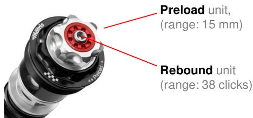
Single hydraulic cartridge kit that completely replace all the existing original fork internals (right side fork only), allowing a full control and adjustment of **Rebound** and **Preload**.
